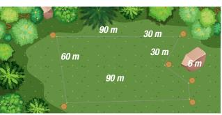
This pasture measures 306 m and includes a gate and must also bypass a large boulder. Therefore 6 stable corner posts are needed. For some of the long distances between the posts, line posts should be placed at intervals of 3 m, which keep 3 levels of wide tape at the same height. For a fence length of 300 m you will need 100 line posts, but this does not include the length of the gate (6 m below the boulder here).
