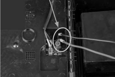
Fig. 4c Connection battery -for 9 VOLT DRY BATTERY or recharging 12V battery Make sure that the polarity is correct!
