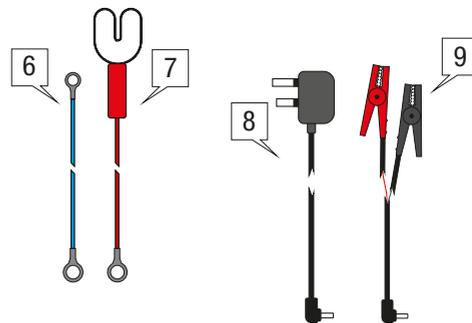
**EN FENCE CONNECTION:** Connect the ring terminals of the earth (no. 6) and fence (no. 7) connection cables to the respective coloured plastic terminals on the energiser (no. 2 and 3) and tighten securely. Then connect the fence and earth connection cables to the conductor material and earth respectively.
